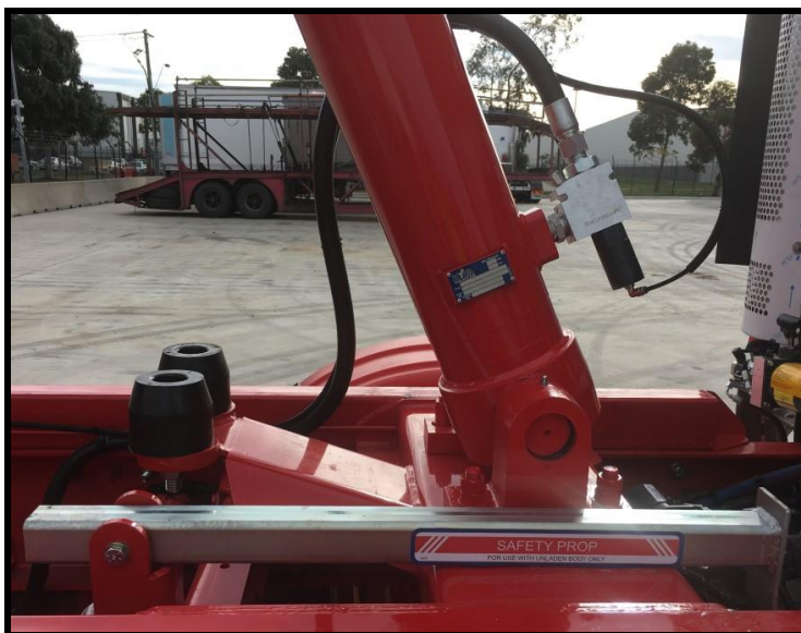
FIGURES 6A: HYDRAULIC BURST PROTECTION CONNECTED TO RAM AND SAFETY PROP LOWERED
